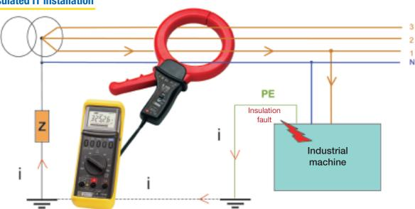
Rugged and very simple to use, the B102 multiple-range current clamp with voltage output can be adapted to any type of multimeter or recorder. It makes preventive measurements, to detect insulation faults. It is a perfect tool for ensuring the conformity of electrical installations to the NF-C 15 100 and CEI 60304 standards. The measurements can
